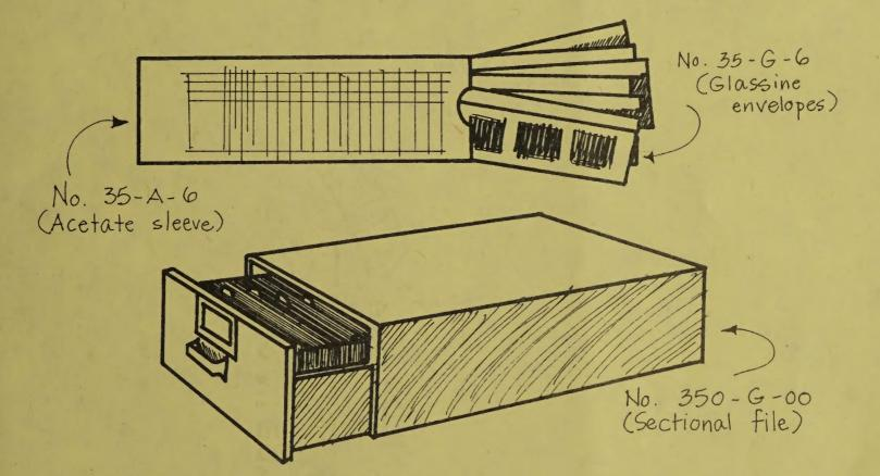
The system provides a means for keeping negatives clean, protection from loss, easy access and identification. The system will be included as an alternative procedure in the forthcoming new manual release on filing procedures.
